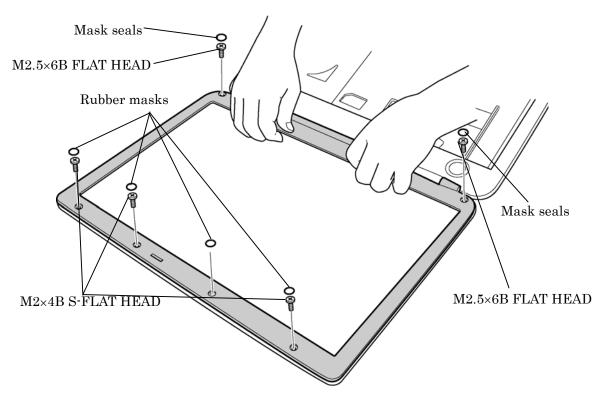
Figure 4-38 Removing the display mask
